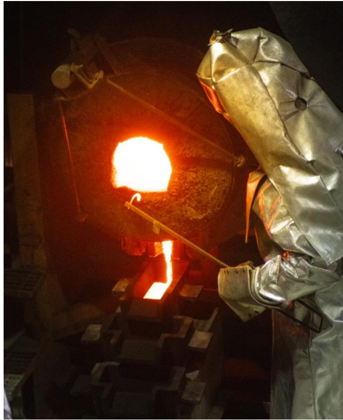
Figure 1: Gold being poured into doré bars at the Borealis ADR facility.
